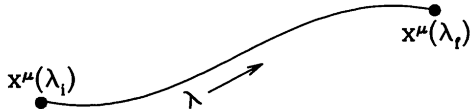
Figure 2.2. A particle's path is parametrized by \lambda , which monotonically increases from its initial value \lambda_i to its final value \lambda_f .
