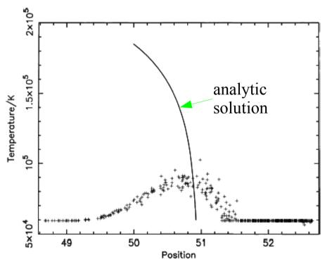
A radiative shock in a shock tube followed with SPH  $t_{cool} \sim h / V_{sh}$
