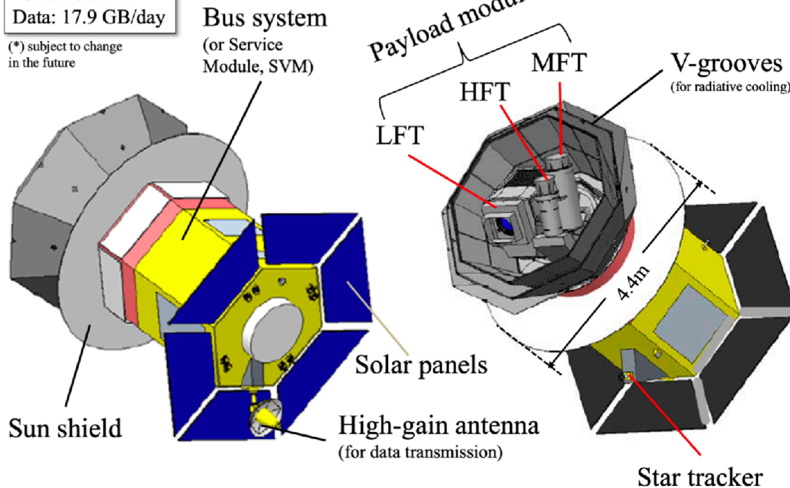
LFT: low frequency telescope
