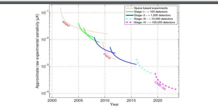
Figure 2. Plot illustrating the evolution of the raw sensitivity of CMB experiments, which scales as the total number of bolometers. Ground-based CMB experiments are classified into Stages with Stage II experiments having O(1000) detectors, Stage III experiments having O(10,000) detectors, and a Stage IV experiment (such as CMB-S4) having O(100,000) detectors. Figure from Snowmass CF5 Neutrino planning locument.
