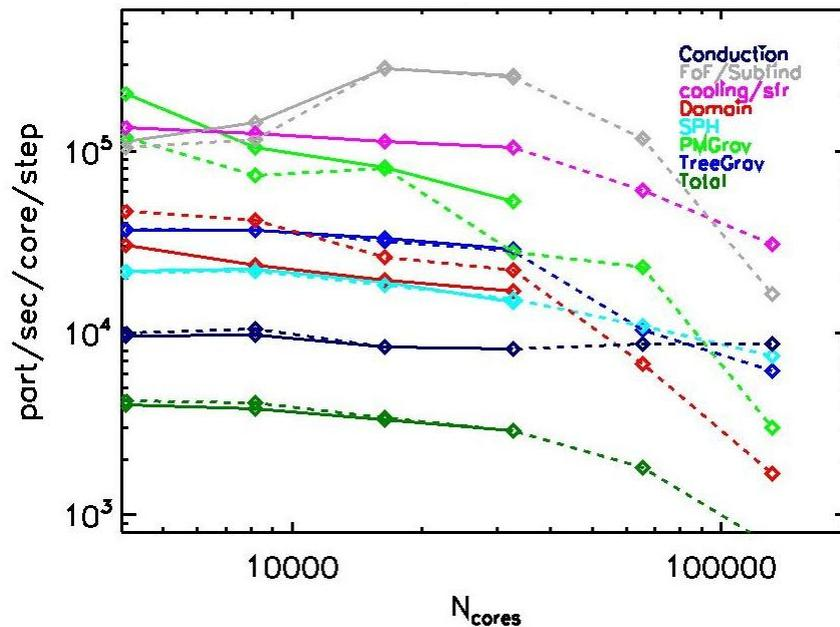
Figure 2 – Strong scaling of Gadget3 on SuperMUC. The plot shows the number of particles processed per core, time step, and wall clock time, measured over the first 10 time-steps, broken down for the most computationally intensive parts of the calculation and spans from 0.5 to 16 islands of SuperMUC. Solid and dashed lines indicate two different communication structures which can be used.
