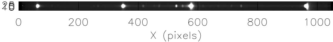
**Figure 2.** Image of the master neon spectra, scaled between 40,000 and 50,000 ADUs for high contrast around the background level to highlight non-circular represents of the fiber on the CCD. The last emission feature appears strongly deformed from unknown reasons.
