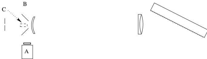
**Fig. 1.** Schematic view of the TRIPPEL spectrograph as seen from above. Components from left to right: entrance slit, pick-off mirrors for ports A-C, field lens, Littrow doublet, grating. Spectral port A has a CCD camera with an interference filter.
