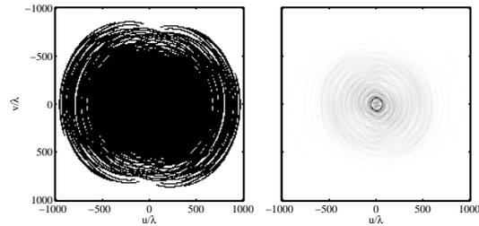
**Figure 2.** Assumed  $uv$  coverage at 150 MHz (left panel): black cells are those containing at least one observation, i.e. those having  $S(u, v) > 0$ . The right panel shows the density of points in the  $uv$  plane, on a linear greyscale.
