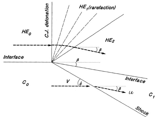
**Fig. 3.** Structure of a detonation propagating at the core–shell interface in the rest frame of the detonation front from Livne & Glasner (1990). (Here the core consists of carbon only, not of C/O like in our case.)
