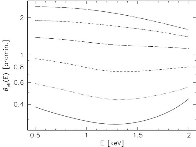
FIG. 2.—Effective radii of the PSPC point-spread function as functions of photon energy, for off-axis angles between  $10'$  and  $60'$  (from bottom to top).
