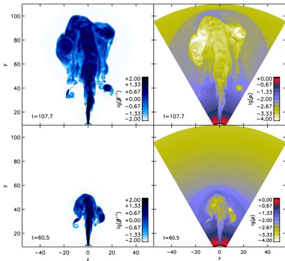
**Figure 2.21:** Slices through a simulated jet, showing the inverse plasma- $\beta$  value (*left*) and the density (*right*) after 77 (*bottom*) and 103 (*top*) rotations at the base. The jet is accelerated into a non-magnetic atmosphere, penetrating through denser material.
