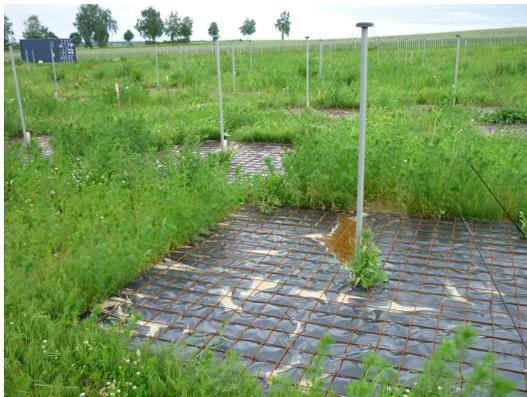
**Figure 1.6:** The LOFAR low frequency antenna field
