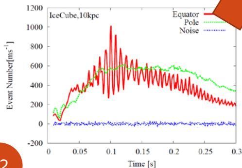
From Frequency of the observed neutrino event, we can extract how high the core rotates at the radius of neutrino sphere.
