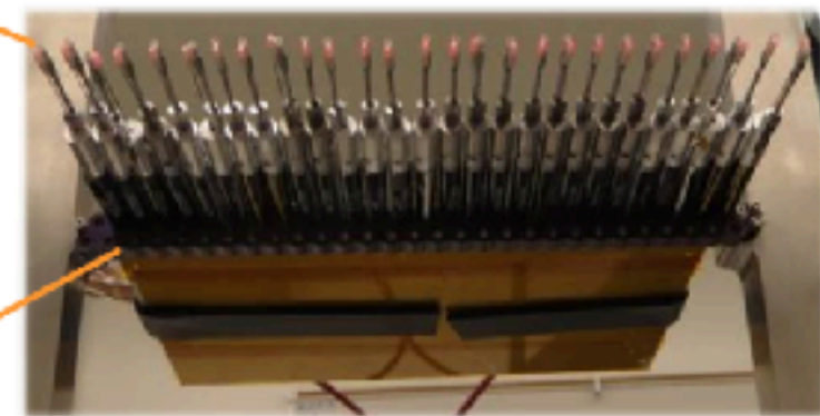
Fiber Positioner "Cobra"
