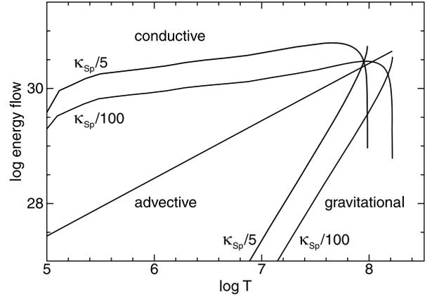
**Fig. 1.** Energy flux versus temperature for heat conductivity 1/5 and 1/100 of the Spitzer value. Note the higher temperature maximum,  $1.6 \times 10^8$  K, for the lower conductivity value.
