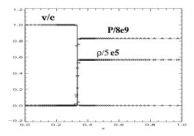
Figure 3. One-dimensional shock heating problem in planar geometry, where a cold fluid hits a wall located at x = 1. The results presented correspond to t = 2. The computational grid consists of 20 zones with 4 levels of refinement. The solid lines are the analytical solution.
