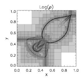
**Figure 4.** Density distribution for the two dimensional shock tube problem at t = 0.4. With a polytropic index  $\Gamma = 5/3$ , a base resolution of  $48 \times 48$  and 4 AMR levels.
