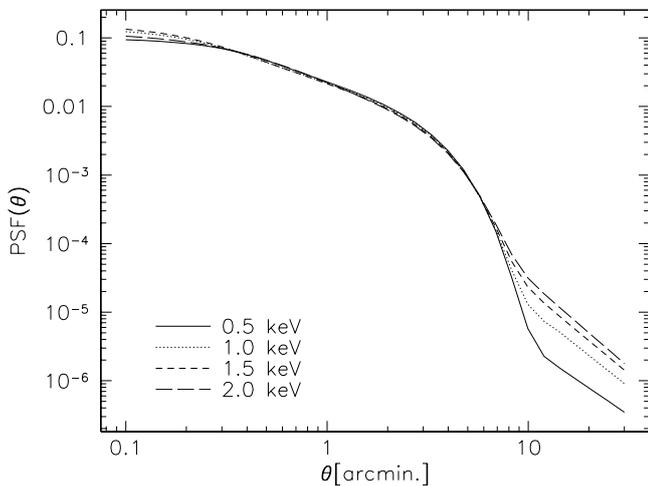
FIG. 3.—The ROSAT-PSPC point-spread function, averaged over off-axis angles within the PSPC field-of-view. The different curves show the point-spread function for four different photon energies, as indicated.
